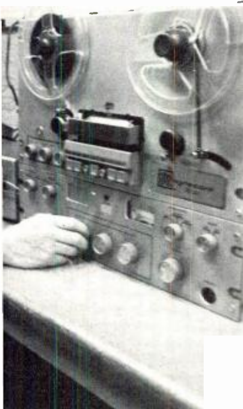
The author using a real time analyzer and a pink noise generator to speed check the frequency response of a tape machine.
